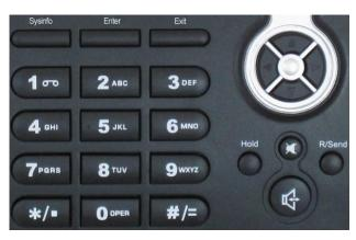
The numeric keypad with the keys 0 to 9, \*, and # is used to enter
